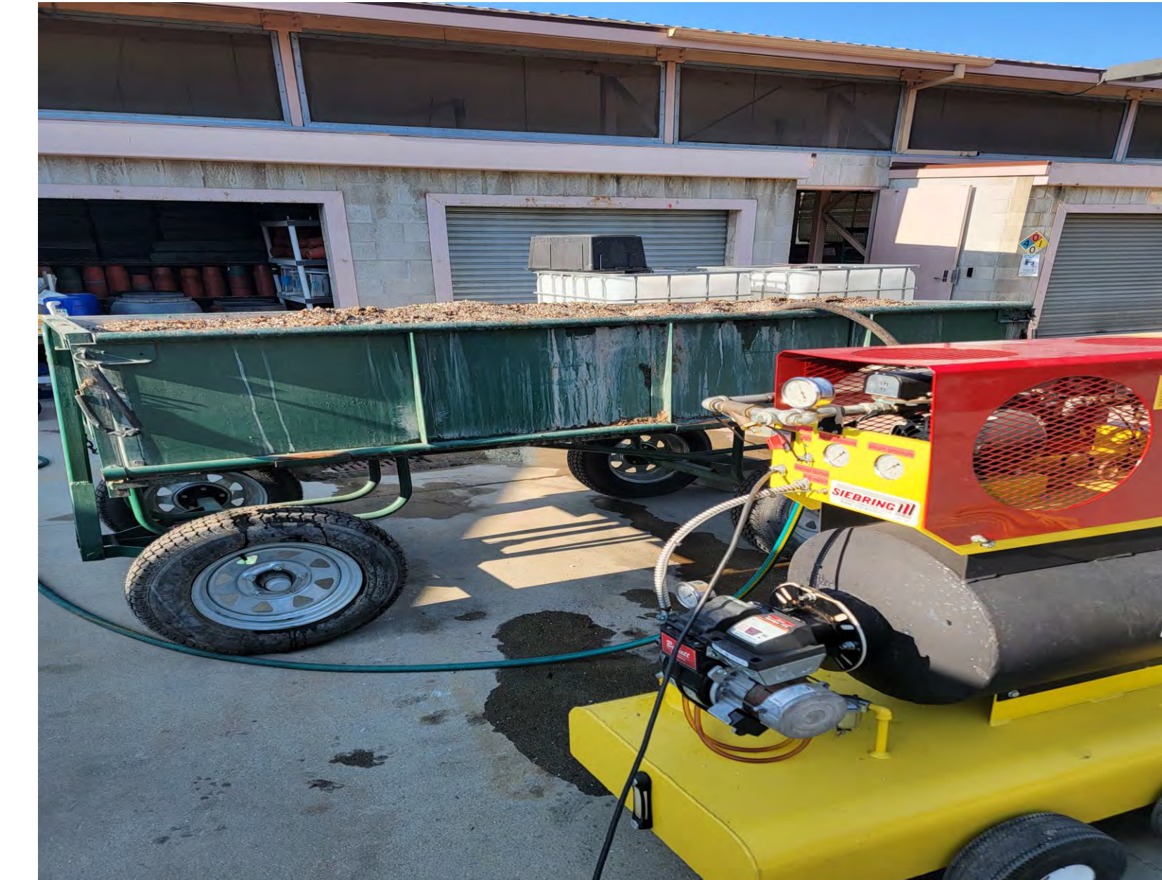
Figure 2. Picture of the soil wagon and steamer at the nursery, sanitizing soil.
