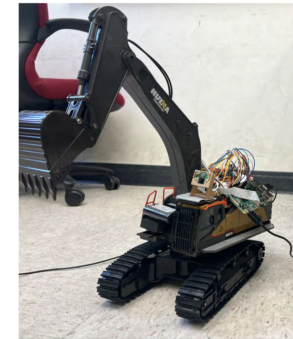
Figure 6: Raspberry Pi controlling toy excavator.
