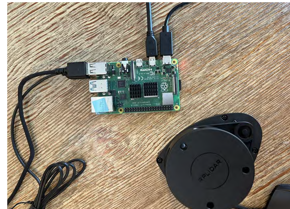
Figure 2: Raspberry Pi 4 attached with RP LiDAR
