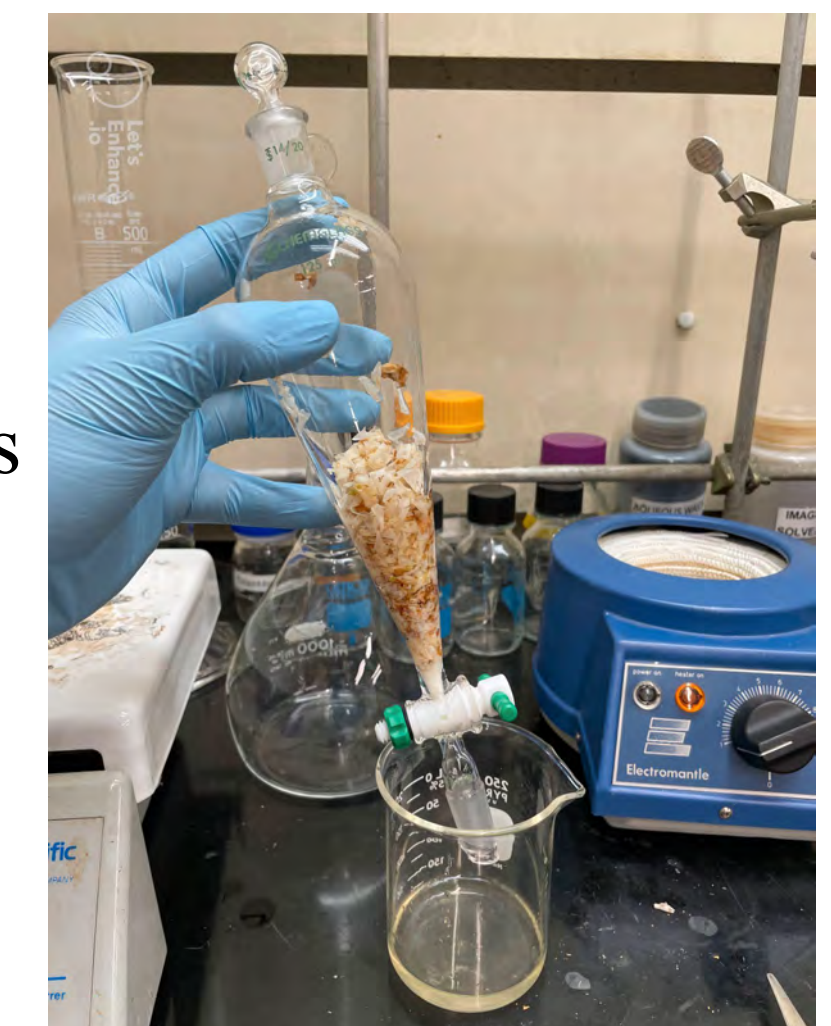
Figure 5: Separatory funnel extraction with untreated flowers.
